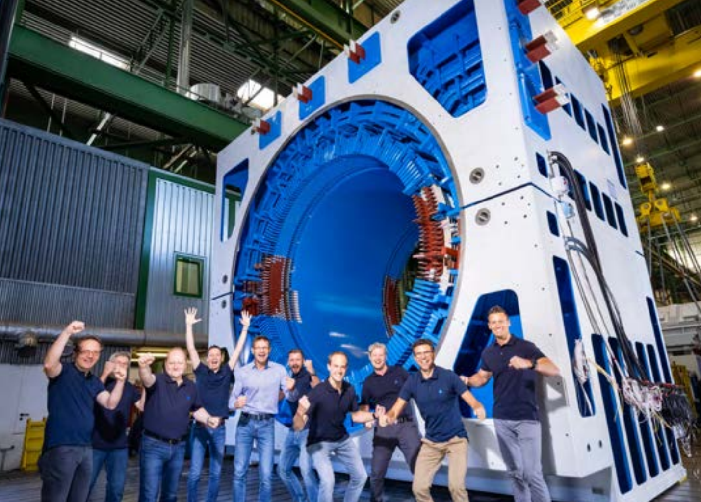
Synchronous condensers are around 400 tons electric machines to safeguard grid stability.
