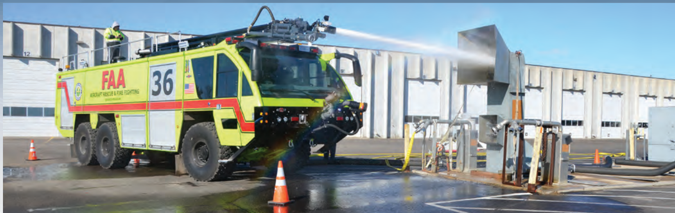
An Aircraft Rescue and Firefighting Vehicle at the Technical Center performing pump pressure and water flow tests to ensure compliance with FAA standards.
