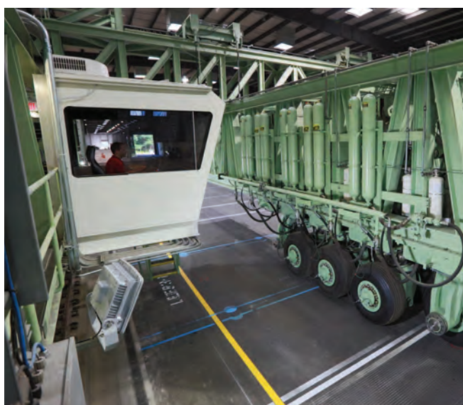
The National Airport Pavement Test Facility, located at the Technical Center, provides high quality, accelerated test data from rigid and flexible pavements subjected to simulated aircraft traffic.
