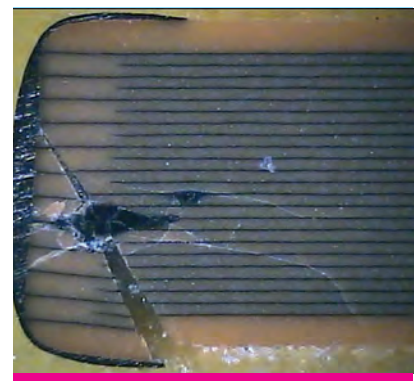
Fig 3: An MLCC that cracked and failed
