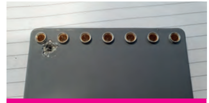
Fig 1: MLCCs failed due to overvoltage
