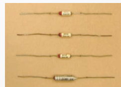
A micro electrolytic capacitor installed in the first model of transistor radio (produced in 1955)
