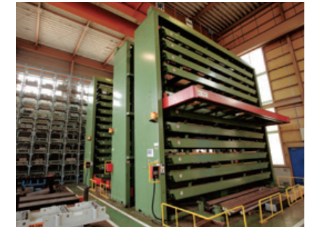
Multilevel automated storage systems
