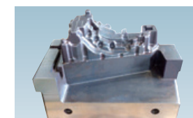
Die-cast intermediate processing (6F+drilling+shaping+heat treatment)
