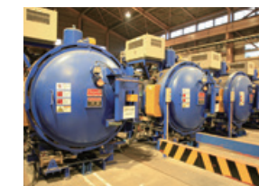
Horizontal pressurized vacuum tempering furnace (Exclusive for high-speed steel)
