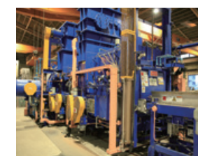
Three-chamber pressure cooling vacuum quenching furnace (Exclusive for high-speed steel)
