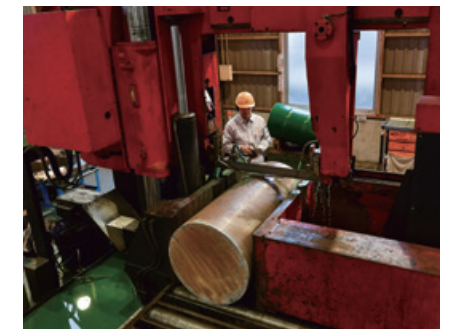
Capable of cutting materials up to 1m in diameter
