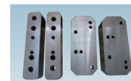
Dies for cold metal sheets (6F+drilling+periphery processing)
