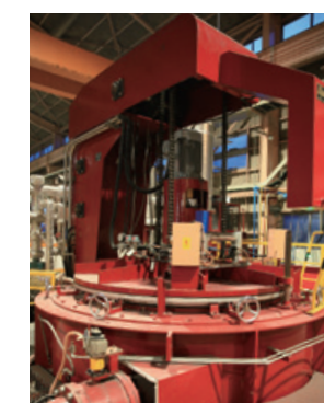
Pit-type gas soft-nitriding furnace
