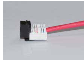
3. The extra wires have to be cut after punching down the wire pairs.
