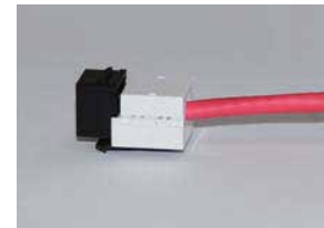
3. The extra wires have to be cut after punching down the wire pairs.
