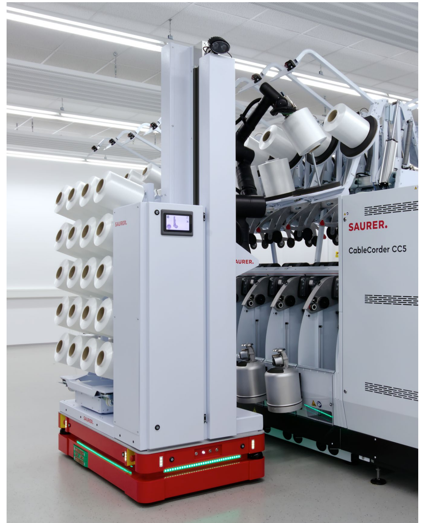
Automatic and autonomous: the Saurer Robot AGV handles and transports cylindrical and conical cross-wound packages.
